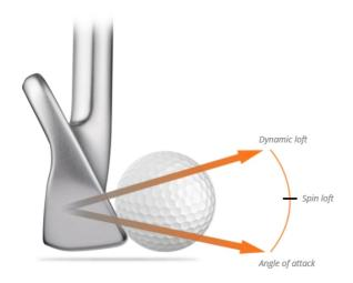
So an attack angle of -4° with a dynamic loft of 38° will create a spin loft of 42°.
